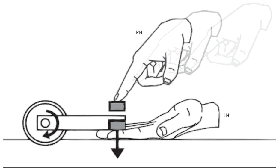
Force is applied to an upper sensor by the index finger on the right hand (RH) and transmitted to the index finger on the left hand (LH) via a sensor mounted on a lever driven by a torque motor. Computerized control of this system manipulated the occurrence and timing of left index finger sensations in both the absence and presence of right index finger movements.
